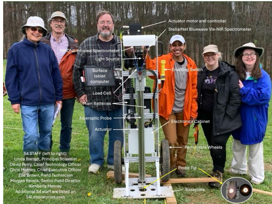
Figure 2. Subterra Grey with labelled parts.
